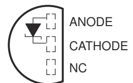
1.2 V . . . LP (TO-92/TO-226) PACKAGE (TOP VIEW)
