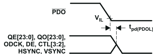
Figure 6-7. Delay From \overline{PDO} Low to Hi-Z Outputs
