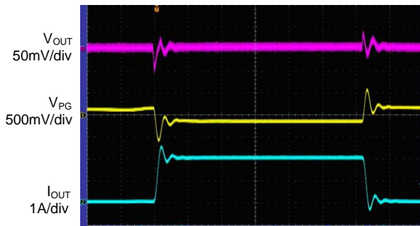
Load Transient ( V_{CTRL}=V_{EN}=5V , V_{IN}=2.2V , I_{OUT}=0 to 2A )
