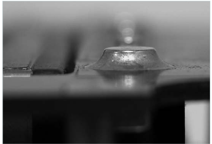
Figure 23.1 — Side profile of a Mini module solder joint
